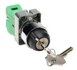
AutomationDirect selector switch, 22mm, 2-position, spring return from right, key removable left position, (1) N.O. contact(s), metal base, metal bezel, Operator: black, key, 30mm, round, plastic.
