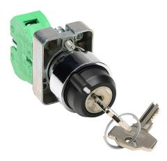
AutomationDirect selector switch, 22mm, 2-position, maintained, key removable in all positions, (1) N.O. contact(s), metal base, metal bezel, Operator: black, key, 30mm, round, plastic.
