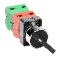
AutomationDirect selector switch, 22mm, 3-position, maintained, (2) N.O./(2) N.C. contact(s), metal base, metal bezel, Operator: black, lever, 30mm, round, plastic.
