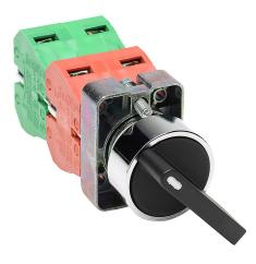
AutomationDirect selector switch, 22mm, 3-position, maintained, (2) N.O./(2) N.C. contact(s), metal base, metal bezel, Operator: black, lever, 30mm, round, plastic.
