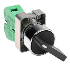
AutomationDirect selector switch, 22mm, 2-position, spring return from right, (1) N.O. contact(s), metal base, metal bezel, Operator: black, lever, 30mm, round, plastic.
