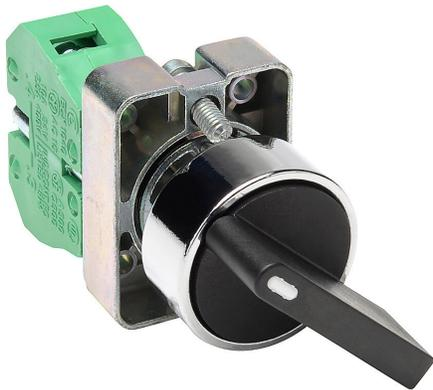
AutomationDirect selector switch, 22mm, 2-position, spring return from right, (1) N.O. contact(s), metal base, metal bezel, Operator: black, lever, 30mm, round, plastic.
