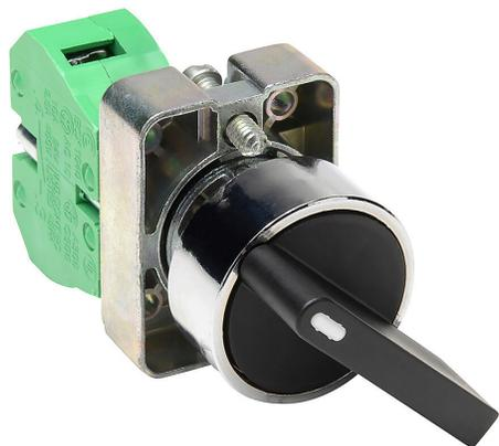
AutomationDirect selector switch, 22mm, 2-position, maintained, (1) N.O. contact(s), metal base, metal bezel, Operator: black, lever, 30mm, round, plastic.
