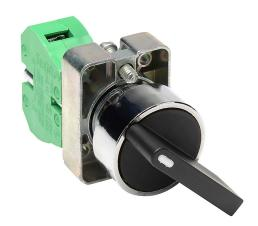
AutomationDirect selector switch, 22mm, 2-position, maintained, (1) N.O. contact(s), metal base, metal bezel, Operator: black, lever, 30mm, round, plastic.
