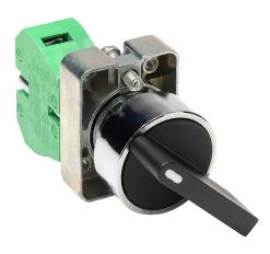
AutomationDirect selector switch, 22mm, 2-position, maintained, (1) N.O. contact(s), metal base, metal bezel, Operator: black, lever, 30mm, round, plastic.
