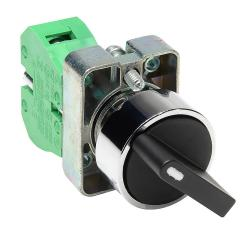
AutomationDirect selector switch, 22mm, 2-position, spring return from right, (1) N.O. contact(s), metal base, metal bezel, Operator: black, knob, 30mm, round, plastic.
