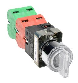
AutomationDirect selector switch, 22mm, 3-position, spring return to center, incandescent illuminated, (2) N.O./(2) N.C. contact(s), metal base, metal bezel, Operator: clear, knob, 30mm, round, plastic, 24 VAC/VDC, full voltage.
