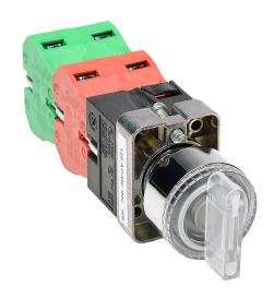
AutomationDirect selector switch, 22mm, 3-position, spring return to center, incandescent illuminated, (2) N.O./(2) N.C. contact(s), metal base, metal bezel, Operator: clear, knob, 30mm, round, plastic, 120 VAC/VDC, full voltage.
