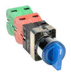
AutomationDirect selector switch, 22mm, 3-position, spring return to center, incandescent illuminated, (2) N.O./(2) N.C. contact(s), metal base, metal bezel, Operator: blue, knob, 30mm, round, plastic, 24 VAC/VDC, full voltage.
