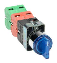
AutomationDirect selector switch, 22mm, 3-position, spring return to center, LED illuminated, (2) N.O./(2) N.C. contact(s), metal base, metal bezel, Operator: blue, knob, 30mm, round, plastic, 24 VAC/VDC, full voltage.
