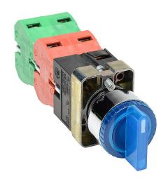
AutomationDirect selector switch, 22mm, 3-position, spring return to center, LED illuminated, (2) N.O./(2) N.C. contact(s), metal base, metal bezel, Operator: blue, knob, 30mm, round, plastic, 120 VAC/VDC, full voltage.
