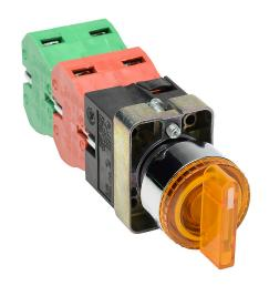
AutomationDirect selector switch, 22mm, 3-position, spring return to center, incandescent illuminated, (2) N.O./(2) N.C. contact(s), metal base, metal bezel, Operator: yellow, knob, 30mm, round, plastic, 24 VAC/VDC, full voltage.
