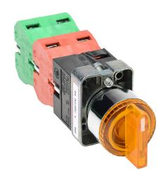
AutomationDirect selector switch, 22mm, 3-position, spring return to center, LED illuminated, (2) N.O./(2) N.C. contact(s), metal base, metal bezel, Operator: yellow, knob, 30mm, round, plastic, 24 VAC/VDC, full voltage.
