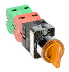
AutomationDirect selector switch, 22mm, 3-position, spring return to center, LED illuminated, (2) N.O./(2) N.C. contact(s), metal base, metal bezel, Operator: yellow, knob, 30mm, round, plastic, 120 VAC/VDC, full voltage.
