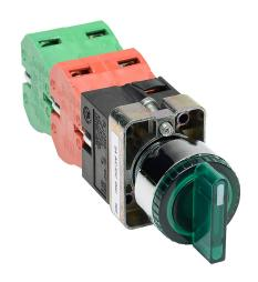
AutomationDirect selector switch, 22mm, 3-position, spring return to center, incandescent illuminated, (2) N.O./(2) N.C. contact(s), metal base, metal bezel, Operator: green, knob, 30mm, round, plastic, 24 VAC/VDC, full voltage.
