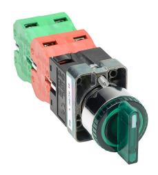
AutomationDirect selector switch, 22mm, 3-position, spring return to center, LED illuminated, (2) N.O./(2) N.C. contact(s), metal base, metal bezel, Operator: green, knob, 30mm, round, plastic, 24 VAC/VDC, full voltage.
