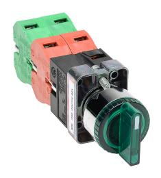
AutomationDirect selector switch, 22mm, 3-position, spring return to center, incandescent illuminated, (2) N.O./(2) N.C. contact(s), metal base, metal bezel, Operator: green, knob, 30mm, round, plastic, 120 VAC/VDC, full voltage.
