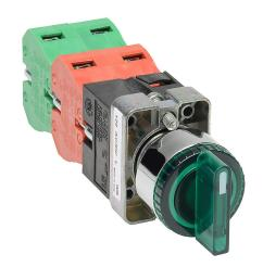
AutomationDirect selector switch, 22mm, 3-position, spring return to center, LED illuminated, (2) N.O./(2) N.C. contact(s), metal base, metal bezel, Operator: green, knob, 30mm, round, plastic, 120 VAC/VDC, full voltage.
