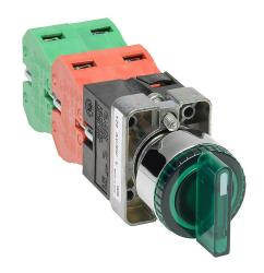
AutomationDirect selector switch, 22mm, 3-position, spring return to center, LED illuminated, (2) N.O./(2) N.C. contact(s), metal base, metal bezel, Operator: green, knob, 30mm, round, plastic, 120 VAC/VDC, full voltage.
