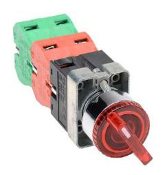
AutomationDirect selector switch, 22mm, 3-position, spring return to center, incandescent illuminated, (2) N.O./(2) N.C. contact(s), metal base, metal bezel, Operator: red, knob, 30mm, round, plastic, 24 VAC/VDC, full voltage.
