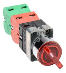
AutomationDirect selector switch, 22mm, 3-position, spring return to center, incandescent illuminated, (2) N.O./(2) N.C. contact(s), metal base, metal bezel, Operator: red, knob, 30mm, round, plastic, 24 VAC/VDC, full voltage.
