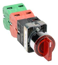
AutomationDirect selector switch, 22mm, 3-position, spring return to center, incandescent illuminated, (2) N.O./(2) N.C. contact(s), metal base, metal bezel, Operator: red, knob, 30mm, round, plastic, 120 VAC/VDC, full voltage.
