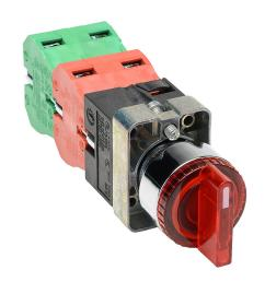
AutomationDirect selector switch, 22mm, 3-position, spring return to center, LED illuminated, (2) N.O./(2) N.C. contact(s), metal base, metal bezel, Operator: red, knob, 30mm, round, plastic, 120 VAC/VDC, full voltage.
