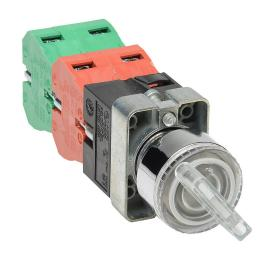
AutomationDirect selector switch, 22mm, 3-position, maintained, incandescent illuminated, (2) N.O./(2) N.C. contact(s), metal base, metal bezel, Operator: clear, knob, 30mm, round, plastic, 24 VAC/ VDC, full voltage.
