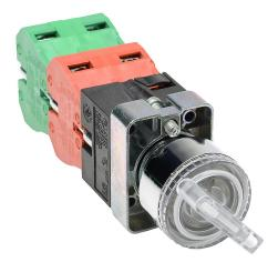
AutomationDirect selector switch, 22mm, 3-position, maintained, LED illuminated, (2) N.O./(2) N.C. contact(s), metal base, metal bezel, Operator: clear, knob, 30mm, round, plastic, 120 VAC/VDC, full voltage.
