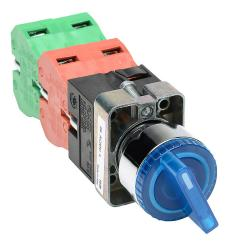
AutomationDirect selector switch, 22mm, 3-position, maintained, LED illuminated, (2) N.O./(2) N.C. contact(s), metal base, metal bezel, Operator: blue, knob, 30mm, round, plastic, 24 VAC/VDC, full voltage.
