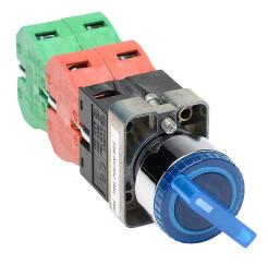
AutomationDirect selector switch, 22mm, 3-position, maintained, incandescent illuminated, (2) N.O./(2) N.C. contact(s), metal base, metal bezel, Operator: blue, knob, 30mm, round, plastic, 120 VAC/VDC, full voltage.
