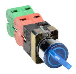
AutomationDirect selector switch, 22mm, 3-position, maintained, LED illuminated, (2) N.O./(2) N.C. contact(s), metal base, metal bezel, Operator: blue, knob, 30mm, round, plastic, 120 VAC/VDC, full voltage.
