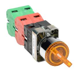
AutomationDirect selector switch, 22mm, 3-position, maintained, LED illuminated, (2) N.O./(2) N.C. contact(s), metal base, metal bezel, Operator: yellow, knob, 30mm, round, plastic, 24 VAC/VDC, full voltage.
