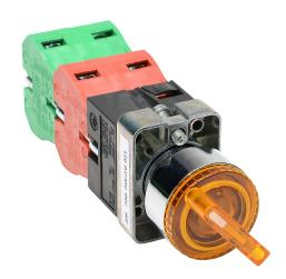
AutomationDirect selector switch, 22mm, 3-position, maintained, incandescent illuminated, (2) N.O./(2) N.C. contact(s), metal base, metal bezel, Operator: yellow, knob, 30mm, round, plastic, 120 VAC/VDC, full voltage.
