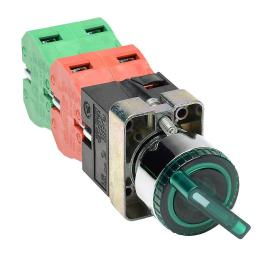
AutomationDirect selector switch, 22mm, 3-position, maintained, incandescent illuminated, (2) N.O./(2) N.C. contact(s), metal base, metal bezel, Operator: green, knob, 30mm, round, plastic, 24 VAC/VDC, full voltage.
