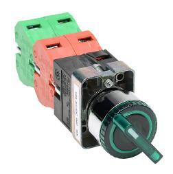
AutomationDirect selector switch, 22mm, 3-position, maintained, incandescent illuminated, (2) N.O./(2) N.C. contact(s), metal base, metal bezel, Operator: green, knob, 30mm, round, plastic, 120 VAC/VDC, full voltage.
