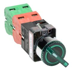
AutomationDirect selector switch, 22mm, 3-position, maintained, LED illuminated, (2) N.O./(2) N.C. contact(s), metal base, metal bezel, Operator: green, knob, 30mm, round, plastic, 120 VAC/VDC, full voltage.
