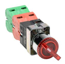
AutomationDirect selector switch, 22mm, 3-position, maintained, LED illuminated, (2) N.O./(2) N.C. contact(s), metal base, metal bezel, Operator: red, knob, 30mm, round, plastic, 120 VAC/VDC, full voltage.
