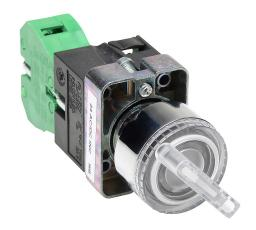
AutomationDirect selector switch, 22mm, 2-position, maintained, incandescent illuminated, (1) N.O. contact(s), metal base, metal bezel, Operator: clear, knob, 30mm, round, plastic, 24 VAC/VDC, full voltage.
