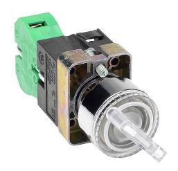
AutomationDirect selector switch, 22mm, 2-position, maintained, LED illuminated, (1) N.O. contact(s), metal base, metal bezel, Operator: clear, knob, 30mm, round, plastic, 24 VAC/VDC, full voltage.
