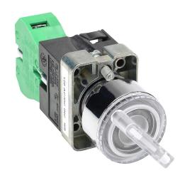
AutomationDirect selector switch, 22mm, 2-position, maintained, incandescent illuminated, (1) N.O. contact(s), metal base, metal bezel, Operator: clear, knob, 30mm, round, plastic, 120 VAC/VDC, full voltage.
