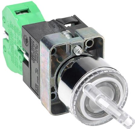
AutomationDirect selector switch, 22mm, 2-position, maintained, LED illuminated, (1) N.O. contact(s), metal base, metal bezel, Operator: clear, knob, 30mm, round, plastic, 120 VAC/VDC, full voltage.
