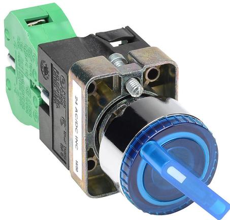
AutomationDirect selector switch, 22mm, 2-position, maintained, incandescent illuminated, (1) N.O. contact(s), metal base, metal bezel, Operator: blue, knob, 30mm, round, plastic, 24 VAC/VDC, full voltage.
