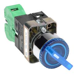
AutomationDirect selector switch, 22mm, 2-position, maintained, incandescent illuminated, (1) N.O. contact(s), metal base, metal bezel, Operator: blue, knob, 30mm, round, plastic, 24 VAC/VDC, full voltage.
