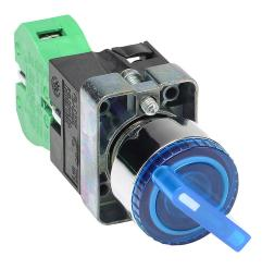
AutomationDirect selector switch, 22mm, 2-position, maintained, LED illuminated, (1) N.O. contact(s), metal base, metal bezel, Operator: blue, knob, 30mm, round, plastic, 24 VAC/VDC, full voltage.
