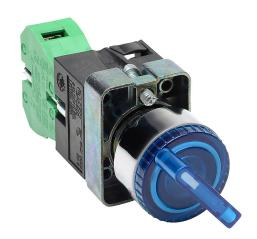
AutomationDirect selector switch, 22mm, 2-position, maintained, LED illuminated, (1) N.O. contact(s), metal base, metal bezel, Operator: blue, knob, 30mm, round, plastic, 120 VAC/VDC, full voltage.
