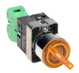
AutomationDirect selector switch, 22mm, 2-position, maintained, incandescent illuminated, (1) N.O. contact(s), metal base, metal bezel, Operator: yellow, knob, 30mm, round, plastic, 24 VAC/VDC, full voltage.
