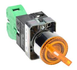
AutomationDirect selector switch, 22mm, 2-position, maintained, LED illuminated, (1) N.O. contact(s), metal base, metal bezel, Operator: yellow, knob, 30mm, round, plastic, 24 VAC/VDC, full voltage.
