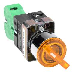
AutomationDirect selector switch, 22mm, 2-position, maintained, incandescent illuminated, (1) N.O. contact(s), metal base, metal bezel, Operator: yellow, knob, 30mm, round, plastic, 120 VAC/VDC, full voltage.
