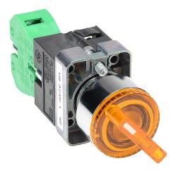
AutomationDirect selector switch, 22mm, 2-position, maintained, LED illuminated, (1) N.O. contact(s), metal base, metal bezel, Operator: yellow, knob, 30mm, round, plastic, 120 VAC/VDC, full voltage.
