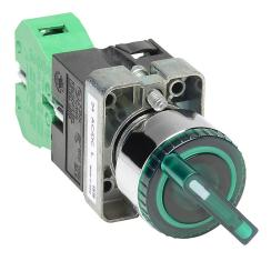
AutomationDirect selector switch, 22mm, 2-position, maintained, LED illuminated, (1) N.O. contact(s), metal base, metal bezel, Operator: green, knob, 30mm, round, plastic, 24 VAC/VDC, full voltage.
