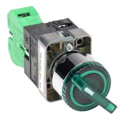
AutomationDirect selector switch, 22mm, 2-position, maintained, incandescent illuminated, (1) N.O. contact(s), metal base, metal bezel, Operator: green, knob, 30mm, round, plastic, 120 VAC/VDC, full voltage.
