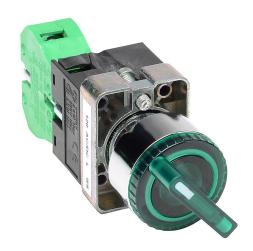
AutomationDirect selector switch, 22mm, 2-position, maintained, LED illuminated, (1) N.O. contact(s), metal base, metal bezel, Operator: green, knob, 30mm, round, plastic, 120 VAC/VDC, full voltage.
