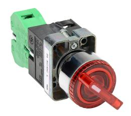
AutomationDirect selector switch, 22mm, 2-position, maintained, LED illuminated, (1) N.O. contact(s), metal base, metal bezel, Operator: red, knob, 30mm, round, plastic, 24 VAC/VDC, full voltage.
