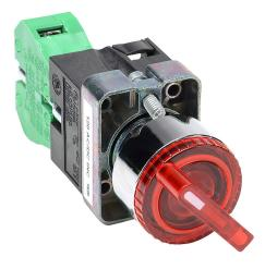
AutomationDirect selector switch, 22mm, 2-position, maintained, incandescent illuminated, (1) N.O. contact(s), metal base, metal bezel, Operator: red, knob, 30mm, round, plastic, 120 VAC/VDC, full voltage.
