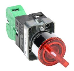
AutomationDirect selector switch, 22mm, 2-position, maintained, LED illuminated, (1) N.O. contact(s), metal base, metal bezel, Operator: red, knob, 30mm, round, plastic, 120 VAC/VDC, full voltage.
