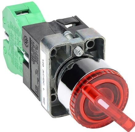
AutomationDirect selector switch, 22mm, 2-position, maintained, LED illuminated, (1) N.O. contact(s), metal base, metal bezel, Operator: red, knob, 30mm, round, plastic, 120 VAC/VDC, full voltage.
