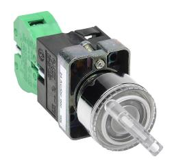
AutomationDirect selector switch, 22mm, 2-position, spring return from right, incandescent illuminated, (1) N.O. contact(s), metal base, metal bezel, Operator: clear, knob, 30mm, round, plastic, 24 VAC/VDC, full voltage.
